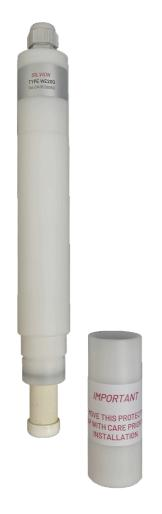
The silver/silver chloride (Ag/AgCl) elements in all Silvion electrodes are manufactured using a "unique" and advanced technique that results in a porous silver matrix. The matrix is then coated with precise quantities of silver/chloride to ensure:
